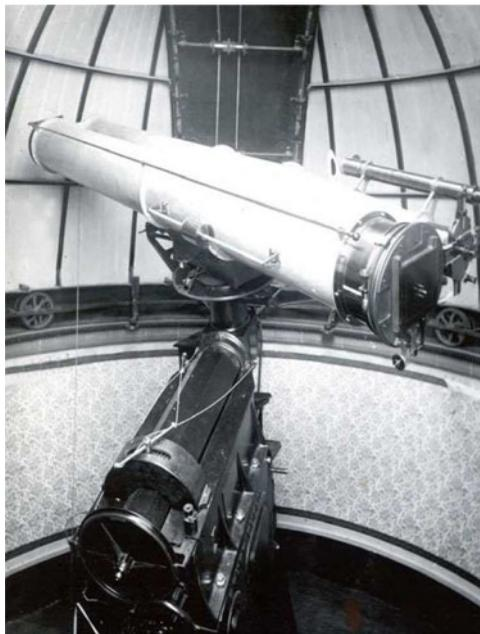
**Figure 6.** Observatory of Tacubaya astrographic telescope, manufactured by H. Grubb (Institute of Astronomy of the National Autonomous University of Mexico).
